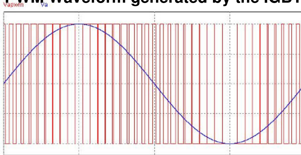
PWM Waveform generated by the IGBT's
